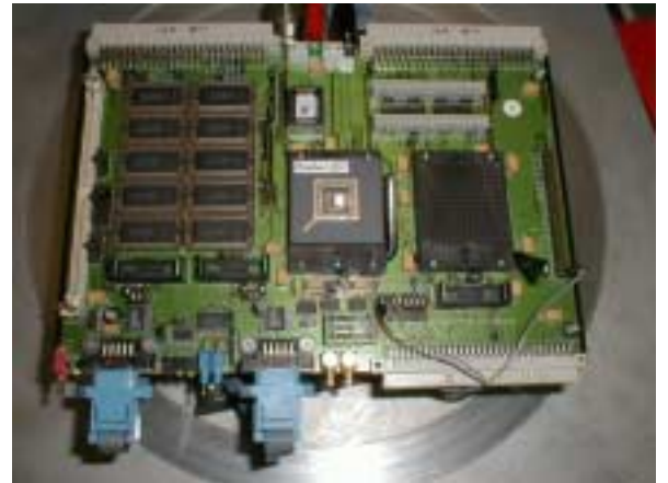
Figure 5: LEON-Express SEU test board
